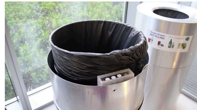
Figure 1. The prototype can be placed inside a trash bin or placed in between the trash can and the plastic bag.
