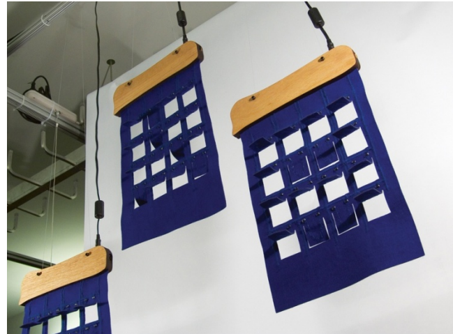
Figure 1. Shutters ' louvers are controlled with a circuit board concealed in the wooden panel. The Shutters on the right has its louvers arranged to display the letter 'A'.
