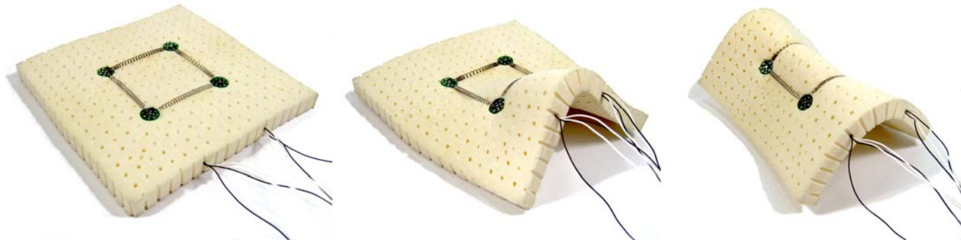
figure 1. Surflex's surface deformation in three steps
