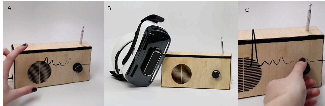
Figure 1. (A) Real time feed from the HMD. The user is performing a gesture to amplify the sound wave of the radio. (B) The system uses a HMD with an embedded depth sensor and a camera to see the real world and overlay AR content. (C) The user can see sound wave parameters change when manipulating the physical radio buttons.
