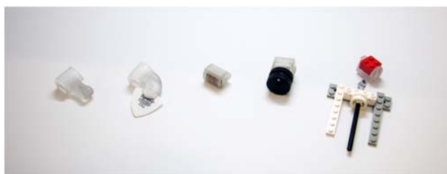
Figure 4: different tip module designs – (from left to right) trigger, pick holder, sensor tip, knob tip, LEGO connector
