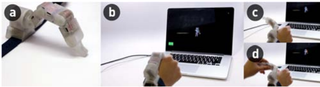
Figure 12: a) gun trigger tip mounted b) the robot used as a gaming interface c-d) running out of ammo triggers a shape change, notifying the user of a required action
