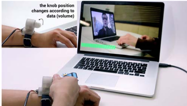
Figure 13: the wearable robot is also an always-available control interface, capable of haptic feedbacks
