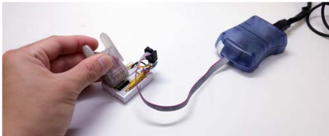
Figure 6: programming a module is done by simply placing the module on a jig connected to an ISP programmer
