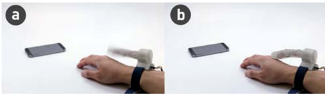
Figure 8: the robot can be used for interpersonal haptic communication – the robot taps on the hand once received a message from a friend or a family member
