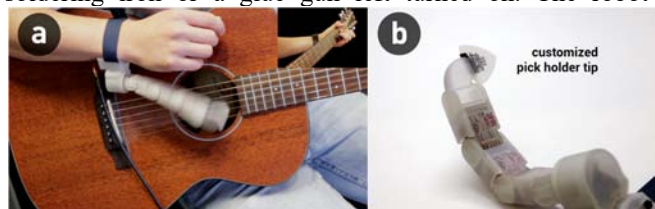
Figure 10: the tip module can be designed to perform variety of operations e.g. holding a pick (b), in turn allowing the robot to instruct a range of physical tasks such as how to play a guitar
