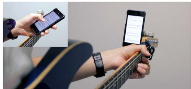
Figure 14: temporarily detached from the user and externally mounted, the robot can give an extra hand
