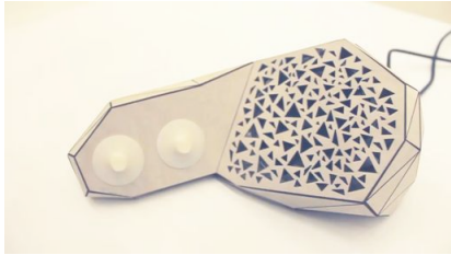
Figure 4: Radio with its TUI represented by a tuner and a volume knob.
