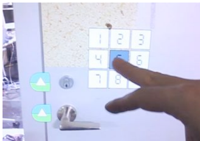
Figure 2: Using an iPad, a User operates a GUI augmented on top of a TUI in order to open a door. Green and blue tags can be seen that represent the components of a door. They can be used to connect the door's functionality with other objects.
